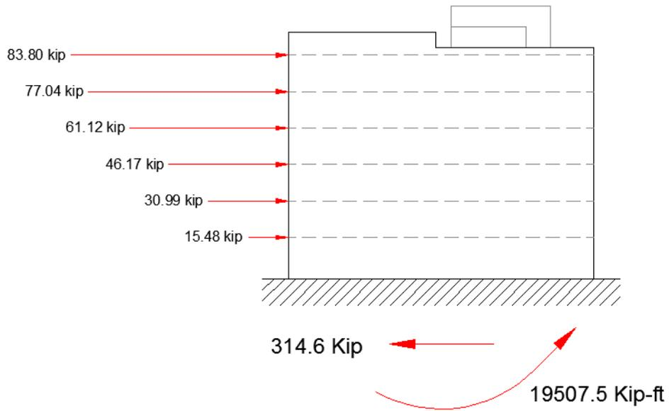
Figure 4.7, Seismic Loads
