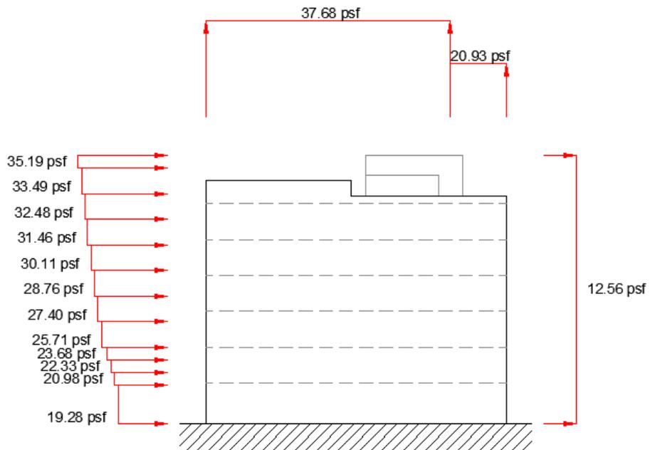
Figure 4.3, MWFRS North/South Wind Load Distribution
