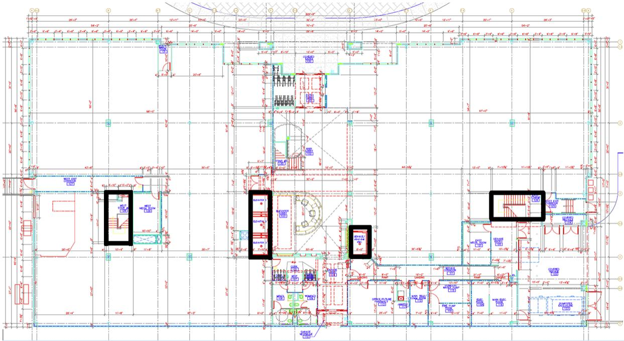
Figure 4.5, Locations of Shear Walls
